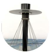
The SAS-2/AB series features extremely broadband omni antennas. These are typically used for lab related testing such as EMC, TEMPEST, etc. Features include Low Noise Amplifiers, a removable monopole, and flexible radials for compact transport and storage. With built in rechargeable batteries, a travel case, and a calibration, these antennas are ready to work in the lab or on the road.
